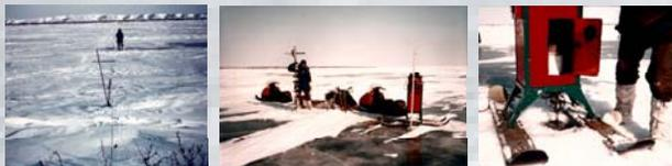
Figure 2. Survey of submarine channels using Wild N2 Engineer's Level and Price WSC Winter Flow Meter.
