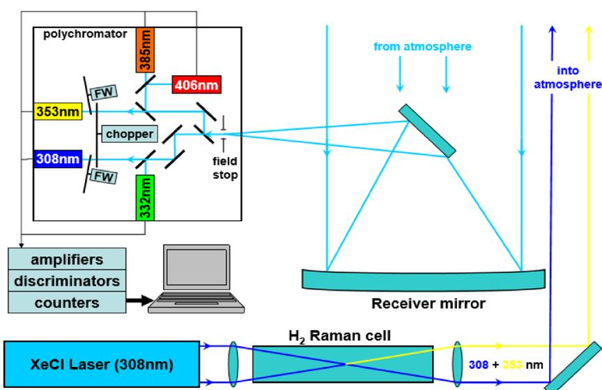
**Figure 1.** The spectral range for the laser beams is chosen in the UV range where one of the wavelengths is highly absorbed by ozone, and is called the on-line wavelength. The other wavelength has a low absorption by ozone and is called the off-line wavelength. Typically, the derivation of the ratio between the on-line and off-line signals is calculated and the ozone density profile is derived.
